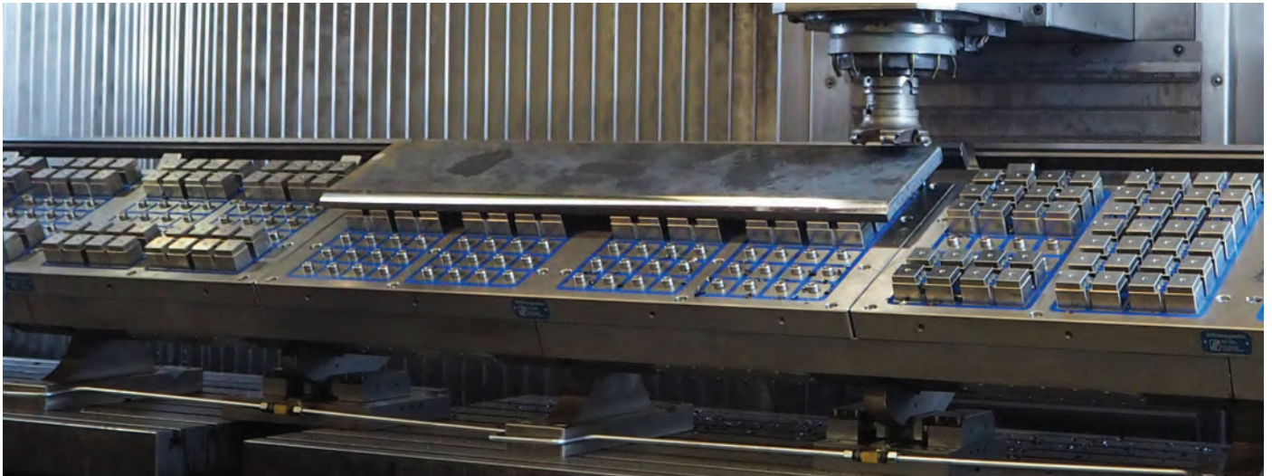
Custom Systems – Magnetic Trunion Table 5,000 x 500 mm (16' x 20"), +/- 45°
